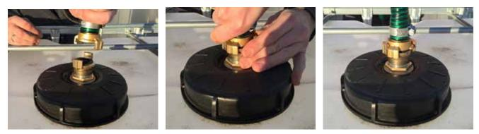
water hose connected to IBC container via quick coupling
